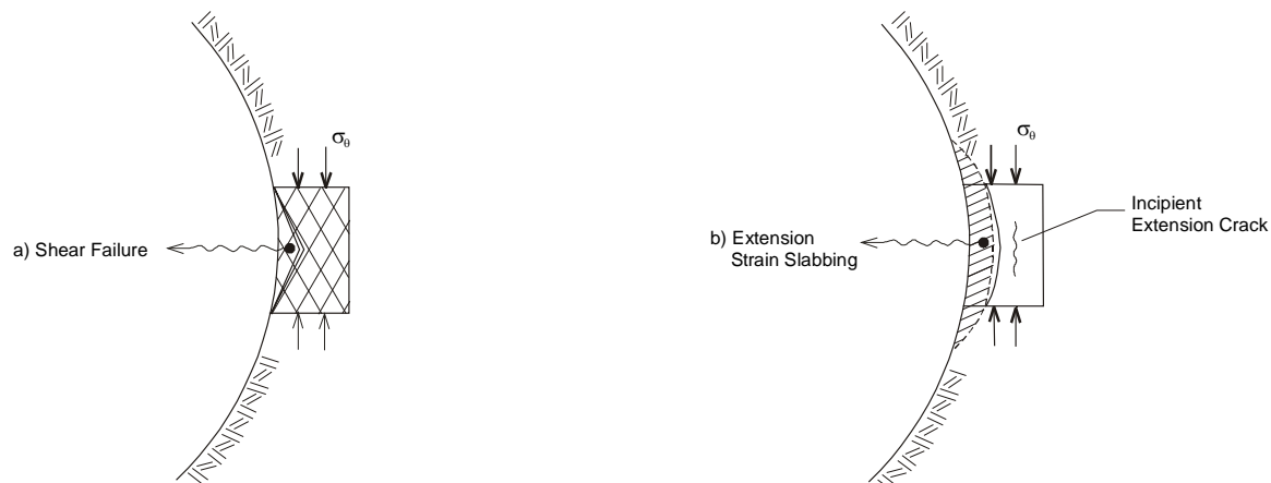
Fig. 6-7 Rock burst in the form of shear failure and 'extension-strain slabbing' in massive rock (from Deere et al., 1969).
