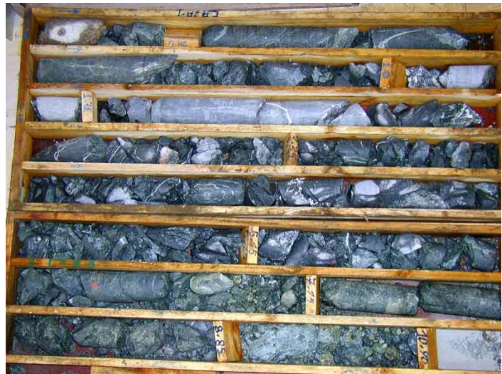
Figure 5: Weakness zone encountered in a core drill hole. There is limited information on the structure of the zone, but in this case the material in the zone has been recovered. Part of the zone contains crushed material, other part (at the end in the box filling of soft material).
