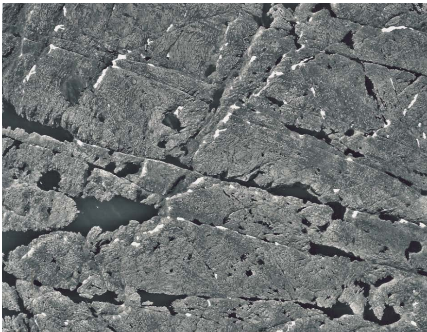
Figure 1: Pattern of weakness zones (and singularities) occurring at the terrain surface. These are seen as distinct lines being more eroded than the surrounding rocks.
