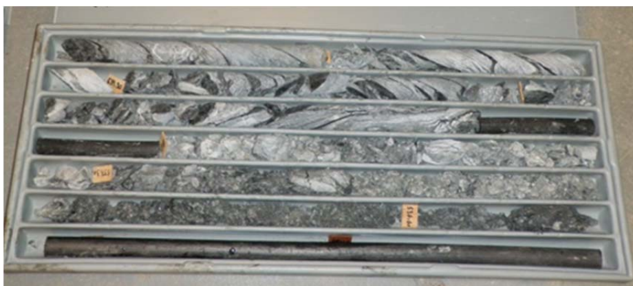
Figure 9. Example of poor quality rock mass from core drilling at Rogfast (black, thinner sections are tubes representing core loss).
