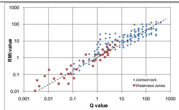
Figure 2. Comparison between the Q and RMI systems
