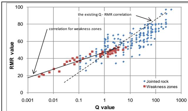
Figure 1. Comparison between the RMR and Q systems
