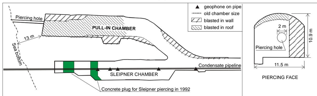
Figure 3: Left: Plan showing areas enlarged in the pull-in chamber from blasting. Right: Cross section of chamber.
