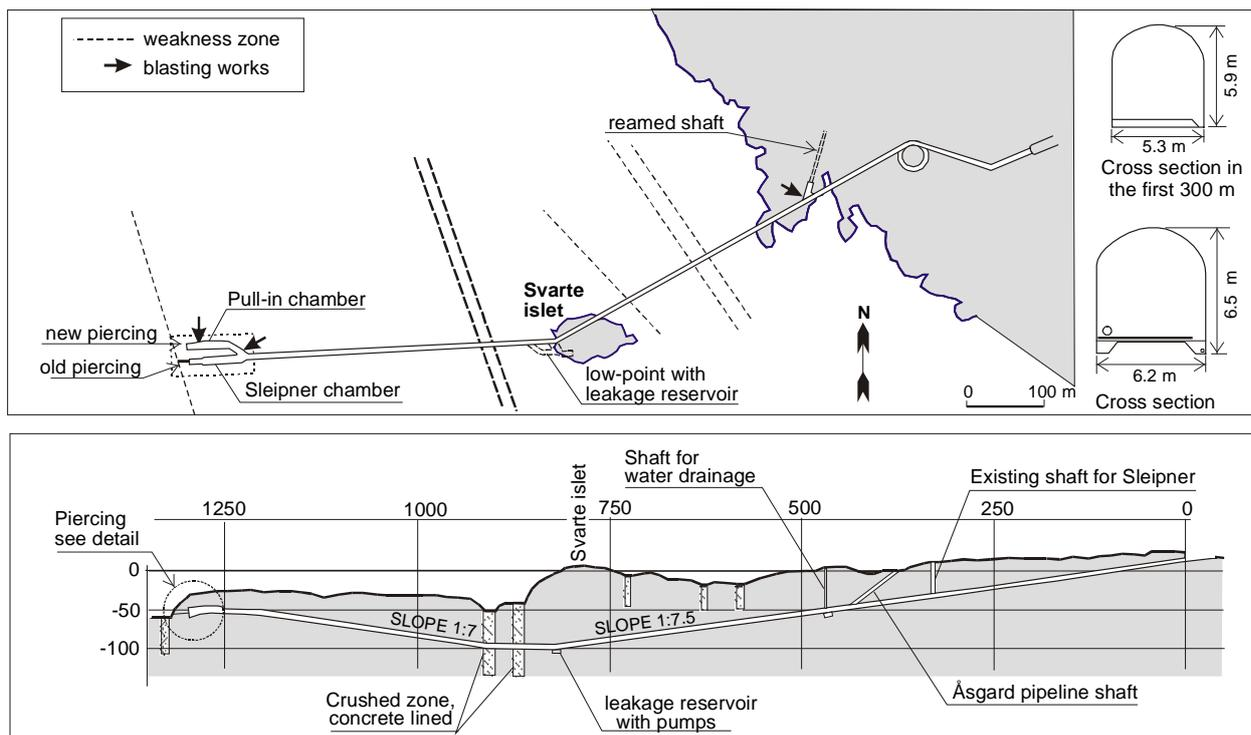
Figure 2: The conditions at the Kalstö landfall tunnel
