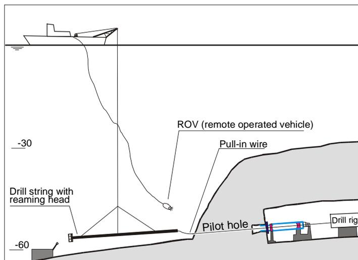
ROVs (remote operated vehicle) equipped with video cameras were used for all sub sea works (connections, inspections, etc.). All sub sea activities was closely monitored in the observation/control centre via TV-links and UHF radio communication (land – sea – tunnel).
