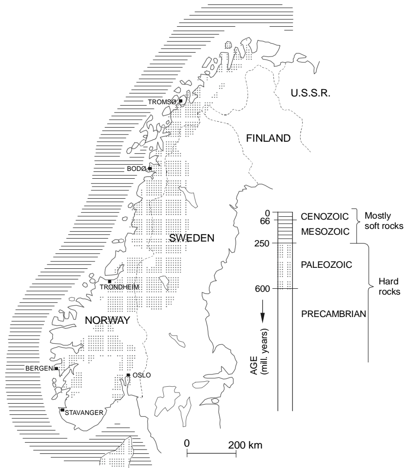
Figure 1 A simplified geological map of Norway. Most of the rocks are older than 250 mill. years. Rocks originally formed as sediments and also many of the plutonic rocks have been metamorphosed to the hard rocks we find today. The most important geological features for underground excavations are joints and faults, which form a complex pattern of discontinuities in the ground.
