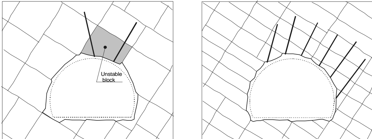
Figure 6 The two main applications of rock bolting. LEFT: Local rock bolts are installed individually to stabilise single, loose blocks. RIGHT: Systematic rock bolts are installed in a certain pattern as a more general support in unstable areas. (In the figure instability is caused by joints shown as lines.)
