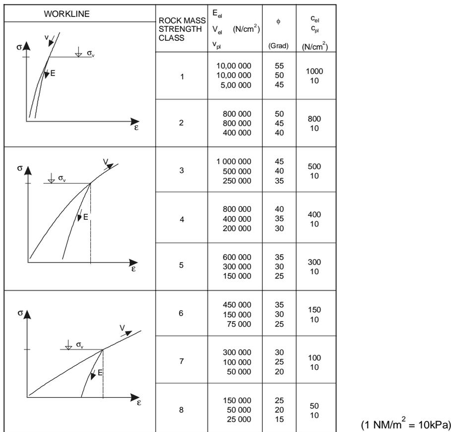
Figure 4. Rock mass strength classes as applied by Seeber et al. (1978)
