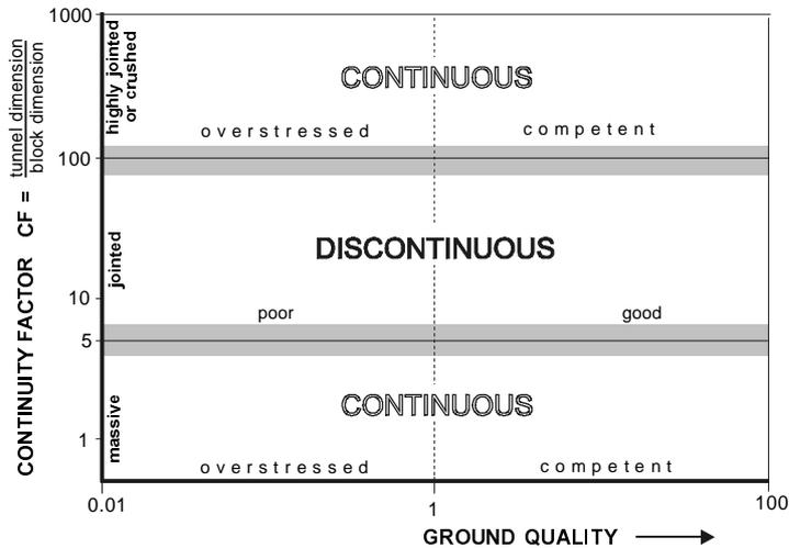
Figure 1 The division of the ground into continuous and discontinuous rock masses. The various groups of ground behaviour are indicated. (from Palmström, 1995a).
