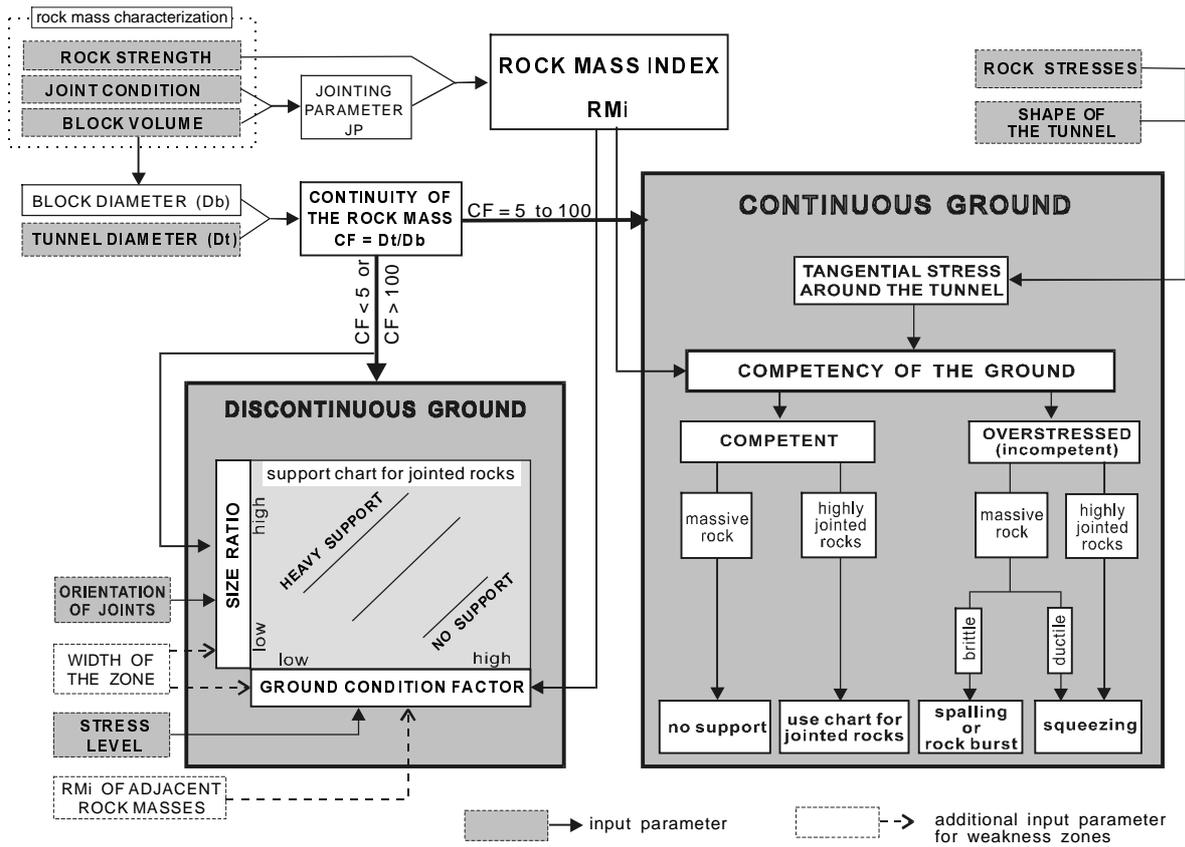
Figure 2 The parameters involved in the RMI method for stability and rock support. For weakness zones the size ratio and the ground condition factor are adjusted for parameters of the zone as indicated. (revised from Palmström, 1995a).
