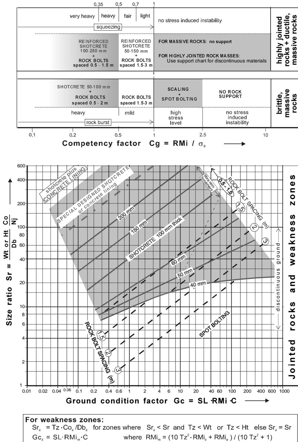
Figure 3. Rock support charts for continuous and discontinuous ground. The support in continuous ground is for tunnels with diameter  $D_t < 15$  m. Note that the diagram for squeezing in particulate materials is based on limited amount of data. (from Palmström, 1995a)
