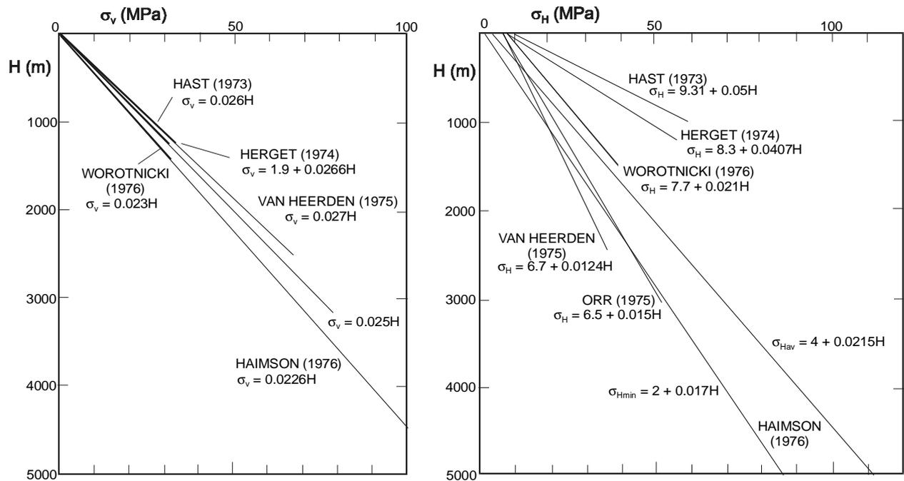
Figure A-1. Vertical and horizontal stresses versus depth below surface according to various authors. Left: Vertical stresses. Right: Horizontal stresses (from Bieniawski, 1984)
