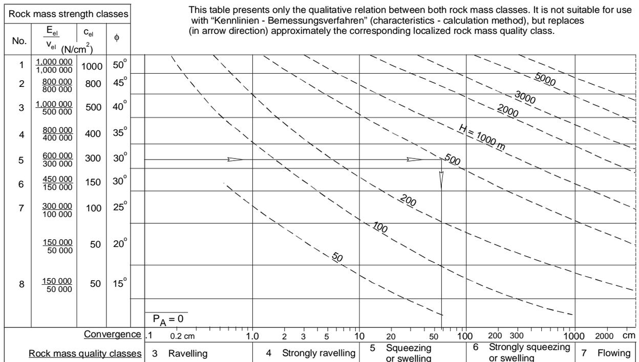
Figure 5 Connection between rock mass strength classes, rock mass quality classes and overburden (from Seeber et al. (1978). Note: Seeber et al. applied an earlier NATM classification of the rock mass quality.
