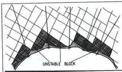
**Fig. 6:** Left: Sprayed concrete (shotcrete), often fibre reinforced, applied for support of unstable rock fragments or smaller blocks (Ref. 12). Right: Combination of rock bolts and shotcrete. The bolts support the larger blocks whilst the shotcrete supports the unstable rock fragments between the blocks (Ref.12).
