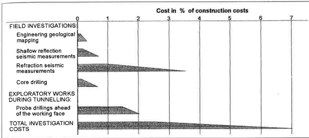
Fig. 4: Approximate distribution of investigation costs for Norwegian subsea tunnels (Ref. 1).
