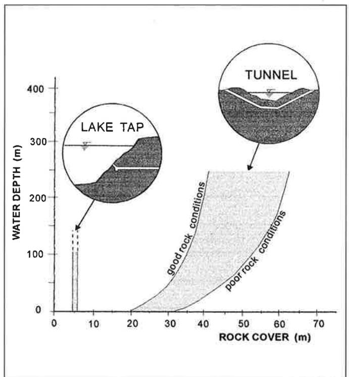
Fig. 1. Minimum rock cover used in Norwegian subsea tunnels.
