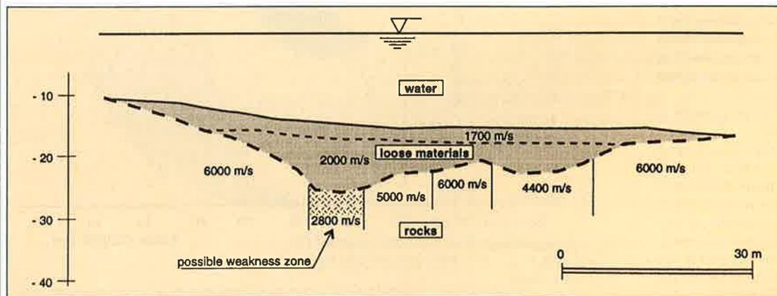
Fig. 2: Example of results from a refraction seismic profile (Ref. 6).
