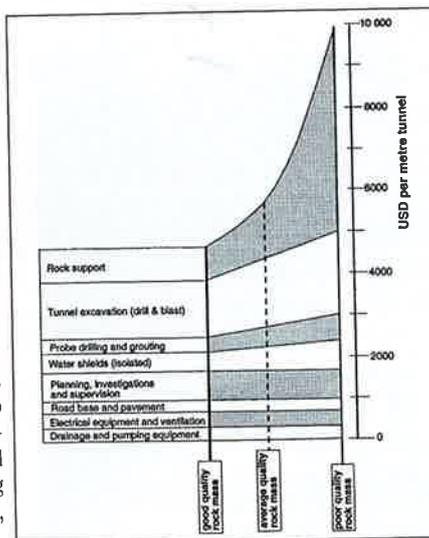
**Fig. 7:** Approximate distribution of total costs for Norwegian two-lane subsea tunnels with 55 m² cross section (Ref. 1).
