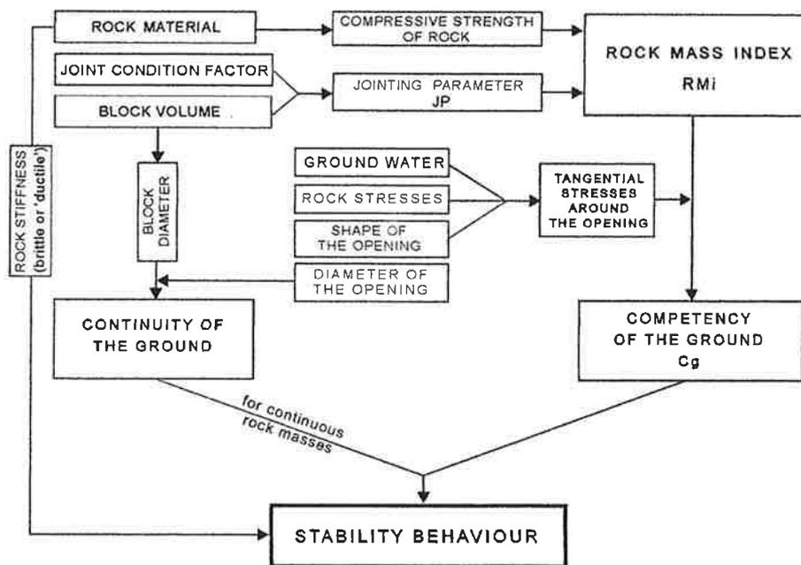
Fig. 1 The principle and the parameters involved in assessment of stability and rock support in continuous rock masses.
