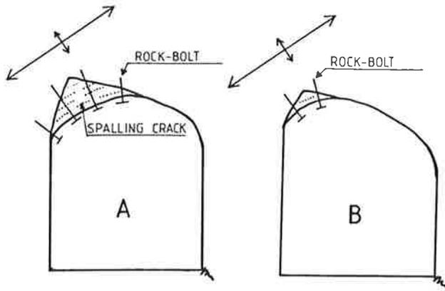
Fig. 4 If high anisotropic stresses occur, the extent of spalling (or rock burst) may be reduced by favourably shaping of the tunnel. 'A' shows the situation in a tunnel with symmetric shape, and 'B' the situation in the tunnel with an asymmetric shape with reduced radius (from Selmer-Olsen 1988)
