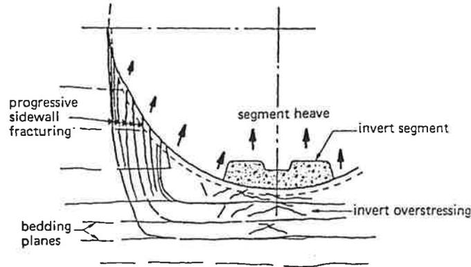
Fig. 6 Example of overstressing mechanism in the lower sidewall and in invert of a tunnel in Cyprus (from Sharp et al., 1993)
