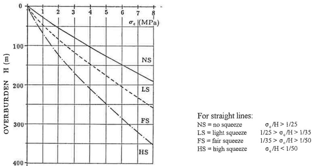
Fig. 7 A chart for estimating the possibility for squeezing (from Aydan et al., 1993)
