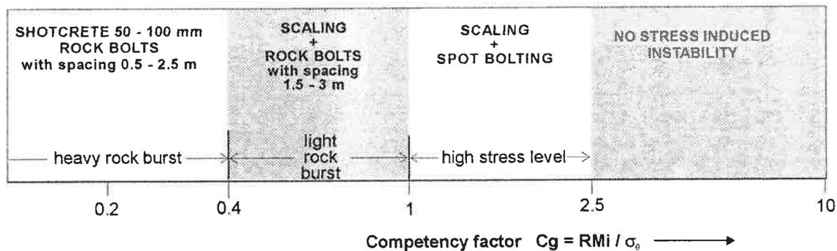
Fig. 3 Relationship between the competency factor, failure modes and rock support in continuous ground of massive, brittle rocks.
