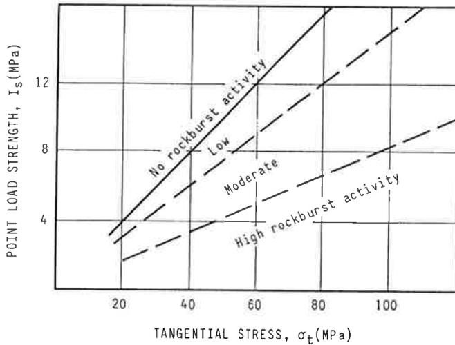
Fig. 2 The level of rock burst related to point load strength of the rock and the tangential stress ( $\sigma_1 = \sigma_\theta$ ) in the tunnel surface calculated from Kirsch's equations (from Nilsen and Thidemann, 1993, based on data from Russenes, 1974).
