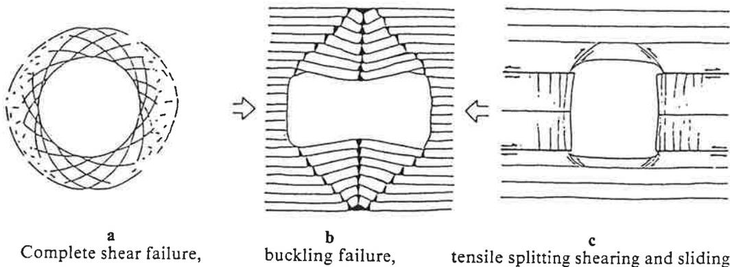
Fig. 5 Main types of failure modes in squeezing ground (from Aydan et al., 1993).
