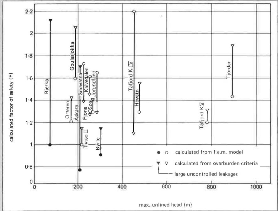
overburden criterion formerly employed against hydraulic splitting. Fig. 2 shows that it indicates a safety factor of less than 1 in respect of certain plants which have suffered such leakage. Had this method been adopted for these plants it would probably have resulted in a different, and safer, location. For this reason the f.e.m. was chosen for the computations required to determine the site of the Tjodan pressure shaft.
