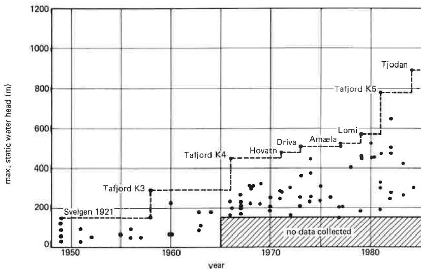
**Fig. 3. Development of pressure shafts/tunnels in Norway.**
