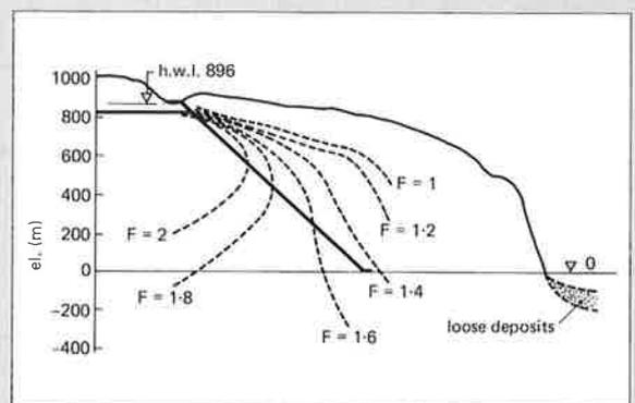
Fig. 6. Safety factors calculated from f.e.m. analysis and rock stress measurements.
