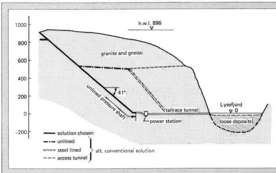
Fig. 9. Two different pressure shaft solutions were evaluated.
