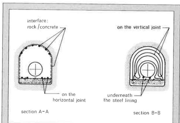
Fig. 11. Typical sections showing the injection hoses before concreting the upper part. (All connection tubes from the injection hoses in the two sections farthest upstream were led to the cone, the rest were led to the penstock chamber).
