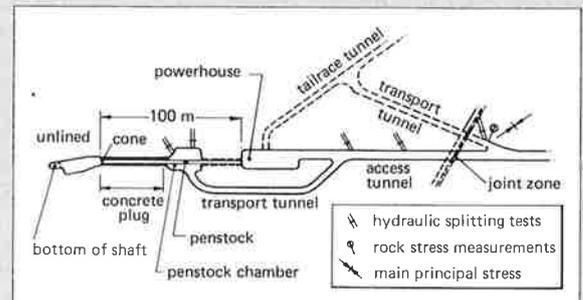
Fig. 5. Locations of rock stress measurements performed in powerhouse area.
