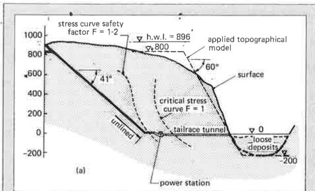
Fig. 4(a) Plan and (b) section of the pressure shaft showing the standard f.e.m. model used.
