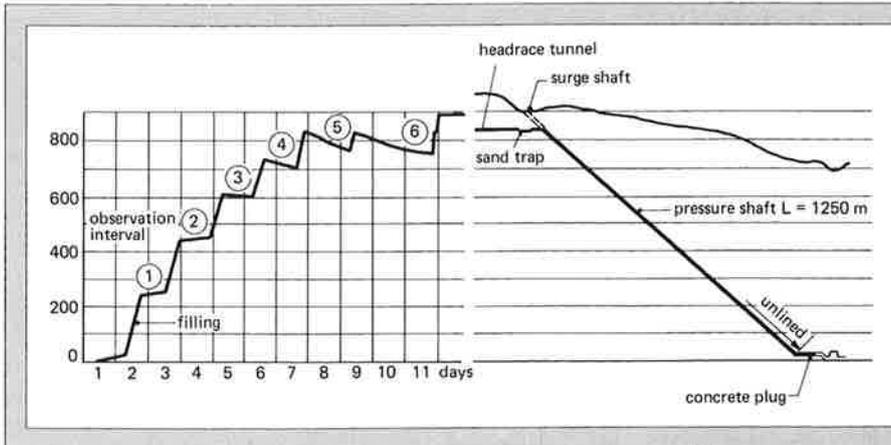
Fig. 7. Filling the pressure shaft in six steps.
