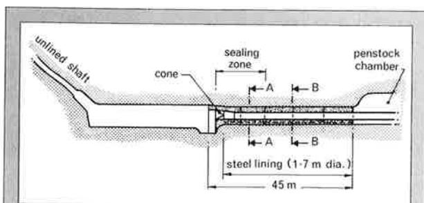
Fig. 10. Concrete plug, longitudinal section.
